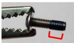
**Loctite Application:** Use one drop about 1 to 2 threads up from the bottom of each screw supplied with the adapter right before installing. (Pictures to the left). Sets in 10 Mins, cures in 24 Hours.
