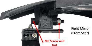
**Step 5:** Attach the PowerMadd Handguards to the mounts using the M6 screw and Nylock nut (No Loctite required). The screw head should be facing toward the rotating adjustment hub. Tighten the nut until it is snug. Do not overtighten.
