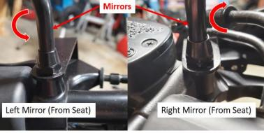
**Step 1a:** Loosen the left mirror nut with a M17 wrench. Loosen CCW. Once the nut is released the mirror also loosens CCW by hand. Remove the mirror. **Do not strip the threads on the mirror or nut.**
