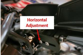
**Step 8:** Move the Universal Mounts to a location that makes both left and right sides equally spaced when viewing from the center. Tighten the M3 screws. Do Not Overtighten.
