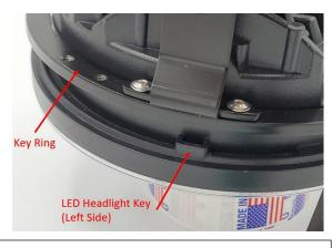
**Step 3:** Take the assembled Key Ring and align the keyway and key of the LED Headlight. Be sure to have the Key Ring sit flush with the headlight.
