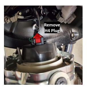
**Step 3:** Remove the Headlight assembly by slightly twisting and pulling on the bezel. Then unplug the H4 plug.
