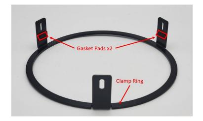
**Step 2:** Apply the two square black gaskets (rubber) to the area pictured (any two tabs). This will eat up any slack between the headlight and the Key Ring. The two tabs pictured should be at the top of the headlight during the next steps.
