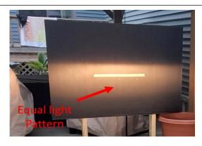
**Adjustment:** After the headlight is installed on your bike position the bike 10 feet from a blank wall. Measure from the ground the height of the headlight (to center) with the rider sitting on it. Now mark your wall with this dimension. Adjust the headlight until the low beam pattern is equally spaced over the line on the wall.
