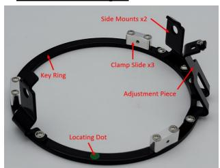
**Step 1:** Take the Key Ring with locating dot facing up and install the two Side Mounts and Adjustment piece using the M3x5 screws. Next install the three metal clamp slides (flat side facing out) using the M3x14 button screws.
