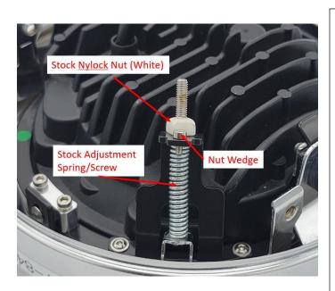
**Step 6:** Now add the stock adjustment spring between the bezel adjustment mount and the Adjustment Piece. Try to align the spring with both holes. *Caution, the spring may launch under load.* **Step 7:** Take the stock M4 long adjustment screw and guide it through the bezel hole and the bezel adjustment hole. Then pass it through the spring. Do not pass it all the way through the Adjustment Piece yet.
