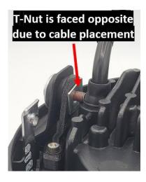
**T-Nut Placement:** You may come across LED Headlights with a wire placement very close to the side mounts. If this is the case flip the T-Nut so that it goes inside the Side Mount hole. This will open up clearance between the LED adapter assembly and the LED cable. Use an M8 Washer (not provided) and place it between the screw and the bezel mount gasket.
