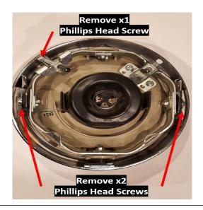
**Step 4:** Remove the adjustment bracket by removing two Philips head screws. Remove one of the adjustment screws from the bezel. Keep the screws, spring and T-Nuts for later use. Keep the grommets in the bezel mounts.
