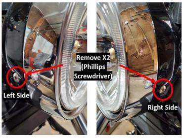
**Step 2:** Next remove 2 Phillips Head screws from the headlight housing connecting the bezel/headlight assembly to the headlight bucket. Be careful not to lose the silver bushings that may fall out.
