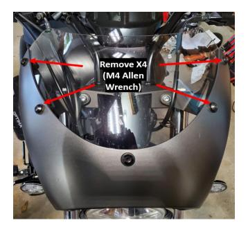
**Step 1 (Optional):** Remove the cowl by removing 4 flat head screws with an M4 Allen wrench. The vibration washers may be free floating, don't lose these.
