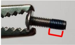
**Loctite Application:** Use one drop about 1 thread up from the bottom of each screw supplied with the adapter right before installing. (Picture to the left). Sets in 10 Mins, cures in 24 Hours.
