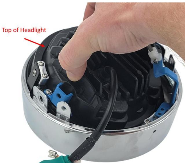
**Step 8:** Slide the LED Headlight Assembly into the Bezel. Position the bottom of the headlight assembly in first getting under the Adjustment Piece. Be careful not to scrape the front face of the Clamp Ring.
